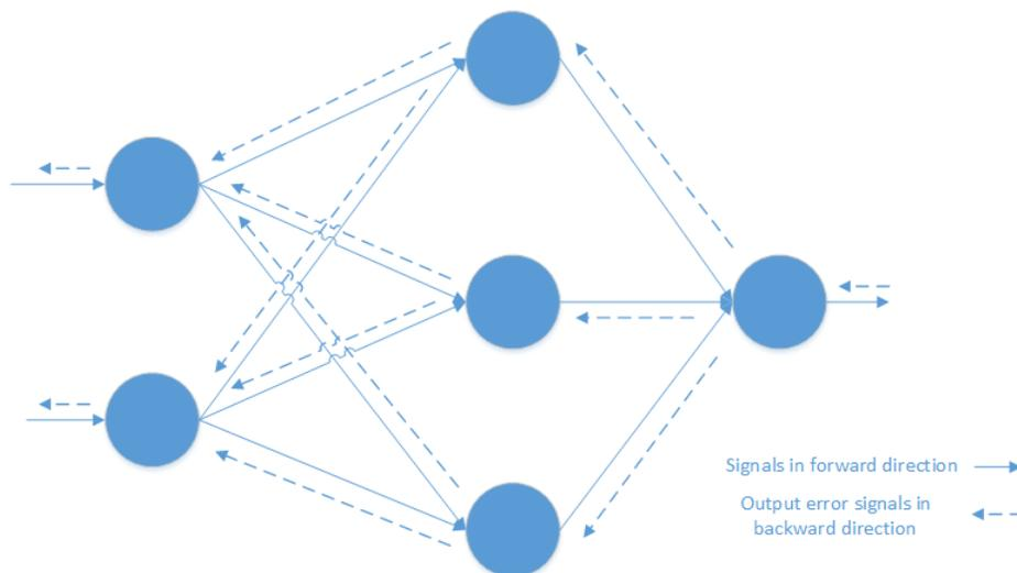
Fig 2. Signal propagation in bp algorithm
